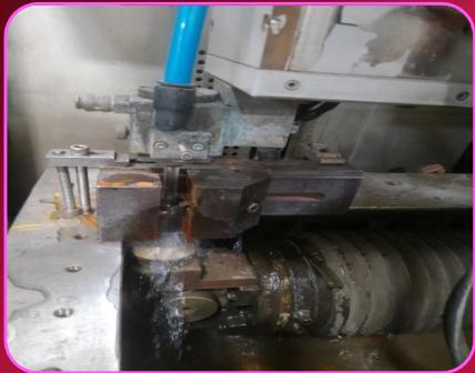
Turning Operation of Cast iron Work pieces
