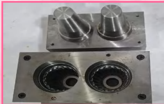
Development of Manufacturing of 2 cavity die set of 200 ml Kulhad
