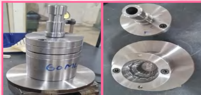
Manufacturing of Single cavity die set for 50 ml & 60 ml Kulhad
