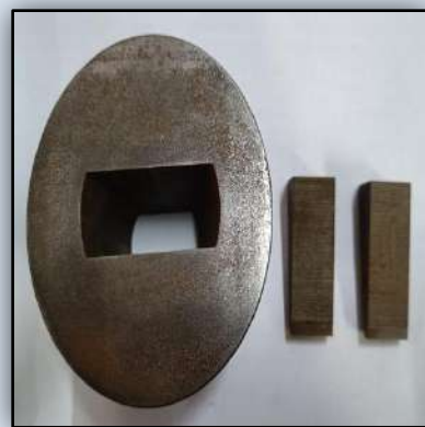
Product Name: CNC Wire-cut EDM Machining of Round Steel B1 Centre: Bhopal
