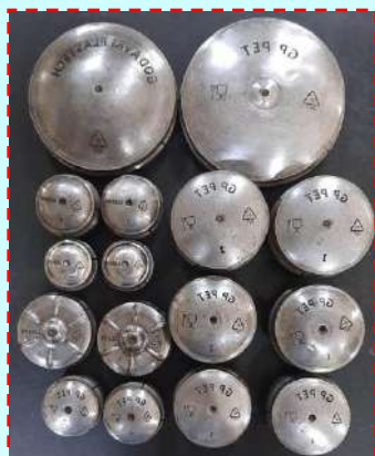
Laser Engraving of PET Bottle/ Jar Mould Bottom Inserts
