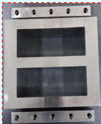
150 x 50 mm (Two Cavity) Die Plate for Ceramic Liner
