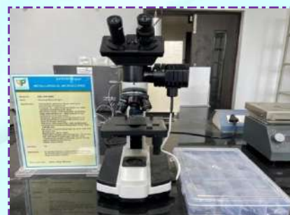
Metallurgical Microscopes Make: Advanced Micro Designs Model: AMD_5000BMM
