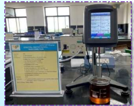
Digital Rotational Viscometer Make: VI Microsystems
