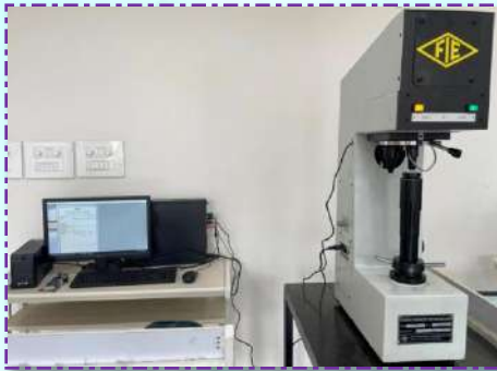
Computerized Vickers hardness testing machine Make: FIE Model: VM 50-PC
