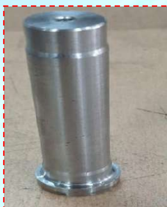
Machining of various Pins in CNC Lathe.
