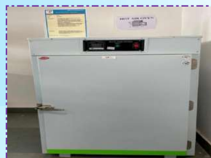
Hot Air Oven Make: SCIENTECH Model: SE-127
