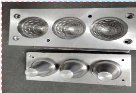
3 Impression Die Set for 70 ml Clay Glass
