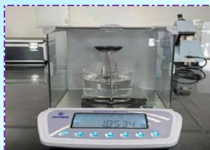
Density Determination Kit Make: Contech Model: CAS-234
