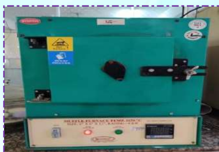
Muffle Furnace Make: SCIENTECH Model: SE-130
