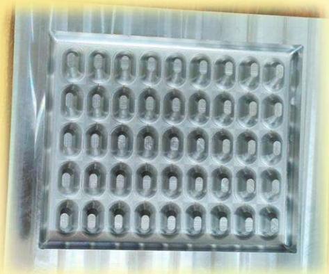
Fabrication of Ventilation Jali mould for (Epoxy materials)
