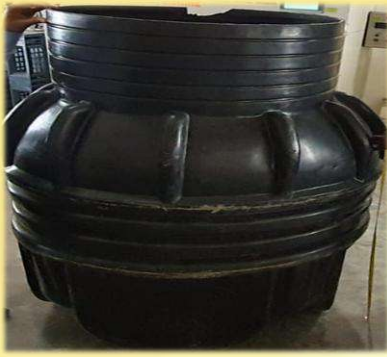
Testing of U Manhole 800 mm as per EN 13598: 2009
