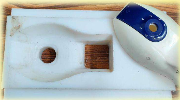
Fabrication of “Bajaj neo wall fan base nylon assembly fixture”
