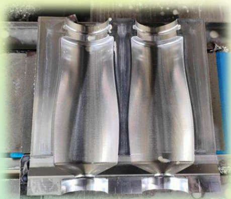
Design & fabrication of 650 ml. shampoo bottle blow mould
