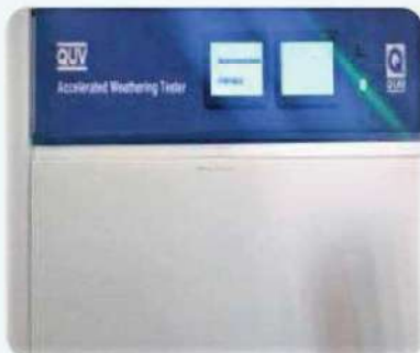
QUV Accelerated Weathering Tester M/s. Q-Lab Corporation Model : QUV/SE model
