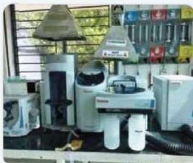
Atomic Absorption Spectroscopy M/s ThermoFisher Scientific Model : ICE 3500
