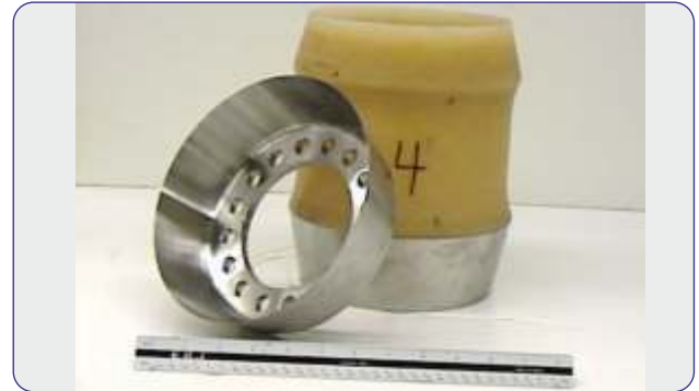
Design & Development of Low Temperature FRP Composite Torque Tube for 200KW HTS Motor for M/s BHEL, Hyderabad.
